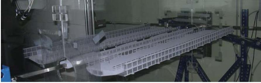
Figure 1: Sectional deck model of the Messina Strait Bridge.
