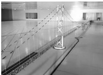
Photo1: Akashi Full-scale Model, 1/100 scale, 40m total span length (courtesy of Honshu-Shikoku BEC)
