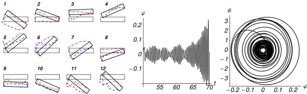
Figure 2. Left: Movement of the beam with large amplitudes during one period. The red (dash-dotted) lines are the pressures on the top surface of the beam. The blue (dashed) line represents the pressures on the bottom face of the body. Pressures pointing out of the body are positive. Right: Response and phase diagram from experiments with increasing velocity. Due to the influence of nonlinear terms, the oscillation has several bumps before the limit cycle oscillation starts.
