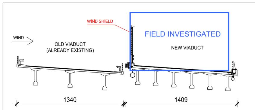
Figure 2. – Bukovo viaduct, made of two bridge decks
