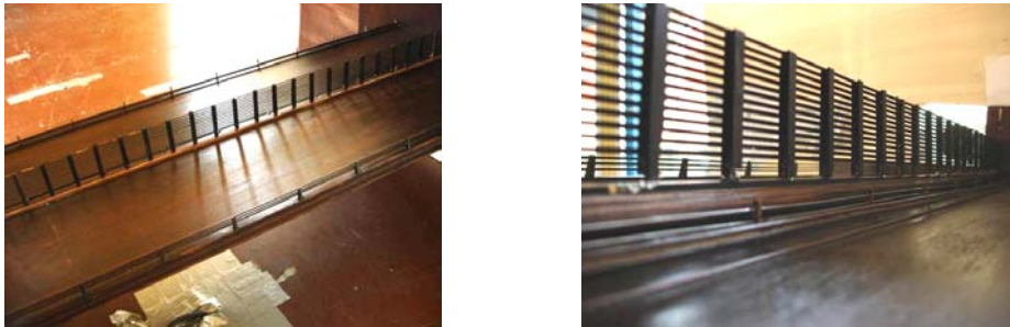
Figure 1. – Wind tunnel model of the viaduct Bukovo
