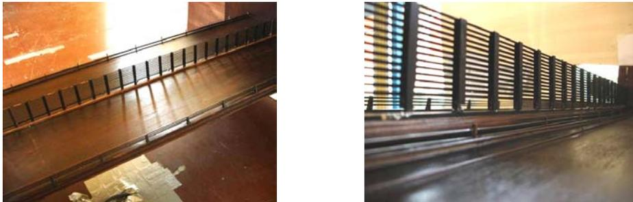
Figure 1. – Wind tunnel model of the viaduct Bukovo
