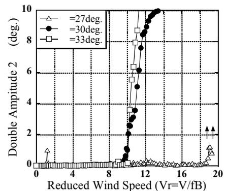
Fig.2 Aerodynamic torsional response at lower plate slope  $\theta=13$ deg.
