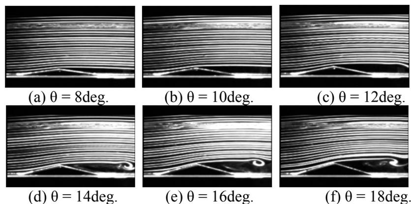
Fig.8 Results of flow visualization
