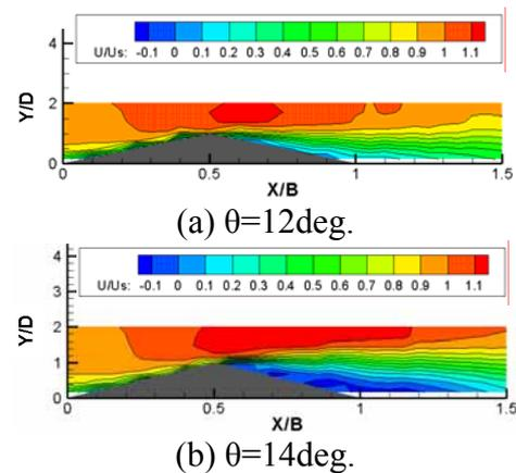
Fig.9 Distribution of mean wind speed ratio of distribution of main flow
