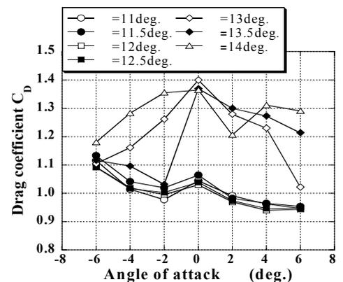
Fig.3 Drag coefficient to angle of attack in  $B/D=5.0$
