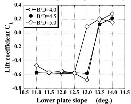
Fig.6 Lift coefficient to Lower plate slope in  $\alpha=0\text{deg.}$
