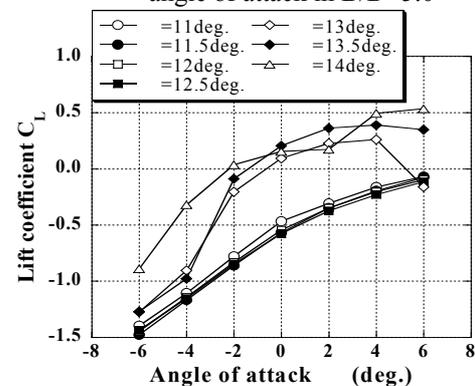
Fig.4 Lift coefficient to angle of attack in  $B/D=0.5$
