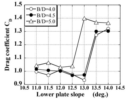
Fig.5 Drag coefficient to Lower plate slope in  $\alpha=0\text{deg.}$
