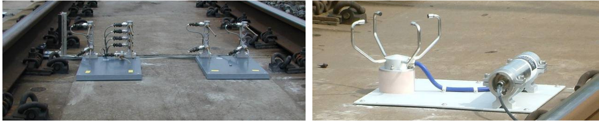
Figure 1: Installation of a Pitot tube rake (left) and of a 2D-Ultrasonic-Anemometer on slab track.
