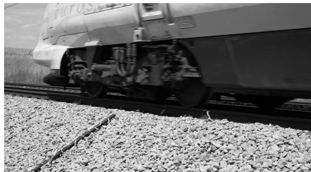
Figure 2 - Photograph of initial observations showing lightweight tapes during a Eurostar pass
