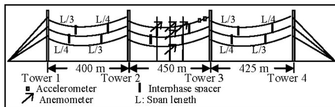
Figure 1: Line setup with interphase spacers
