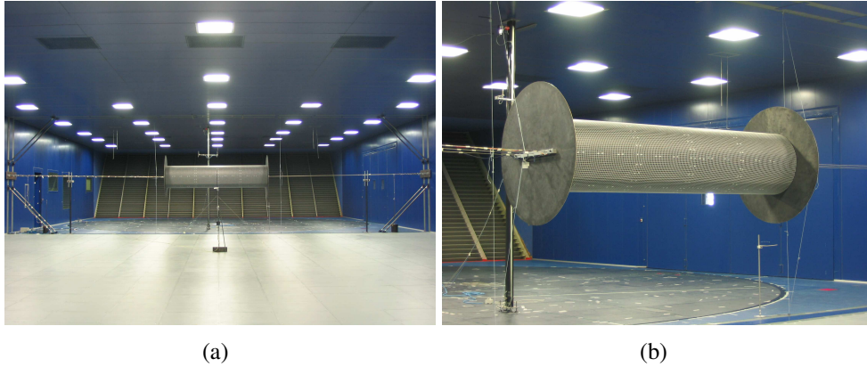
Figure 1: Cylinder model suspended by cables (a) with added surface roughness (b)
