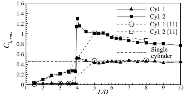
Figure 4: Lift fluctuating force,  $Re=200$ .
