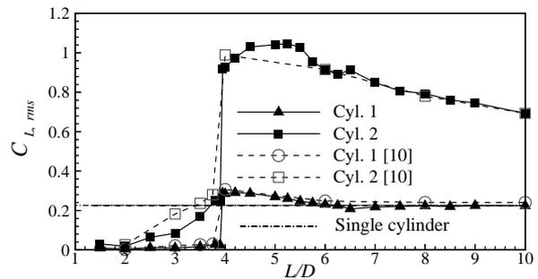
Figure 2: Lift fluctuating force,  $Re=100$ , from [13].
