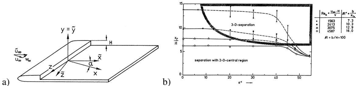
Figure 3: The flow around a swept backward facing step
