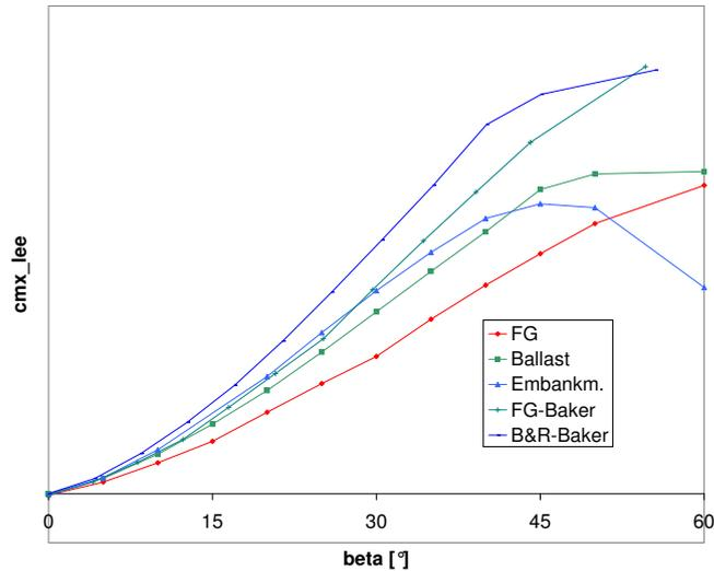
Figure 2: Roll moment coefficient about leeward rail of an ICE 3 on different ground configurations
