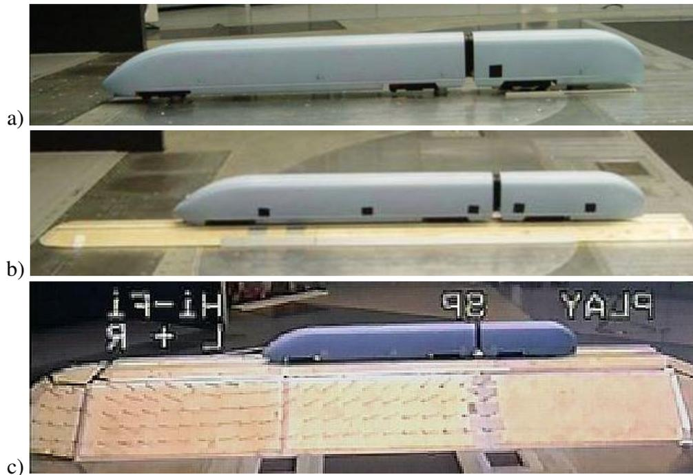
Figure 1: ICE 3 on a) Flat Ground, b) Ballast & rail, c) 6 m Embankment
