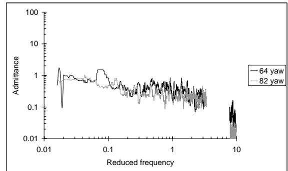
Fig. 3. Side force aerodynamic admittances for the Class 390
