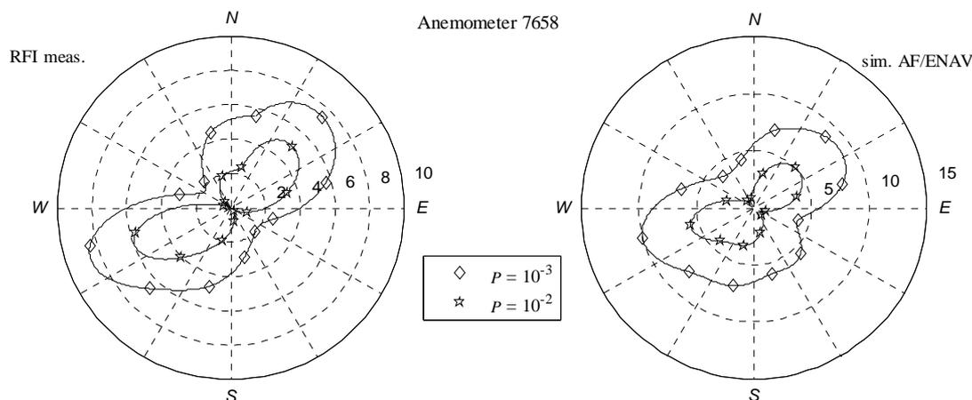
Figure 3: Comparison between the wind velocities with assigned exceedance probability obtained from the analysis of the data recorded along the line (left panel) and those obtained by numerical simulations (right panel).
