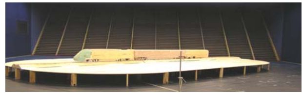
Figure 2. Experimental wind tunnel tests: 1:10 scale model of ETR500 on flat ground with ballast and rail.
