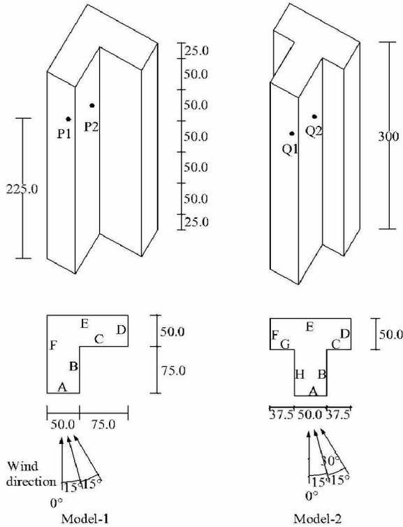
Fig. 1 Plan and isometric view of building models
