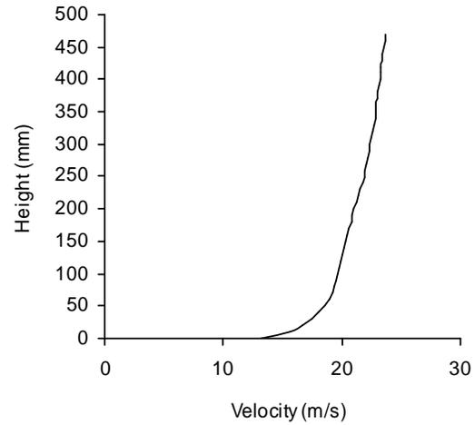
Fig. 2b Velocity profile at the test suction
