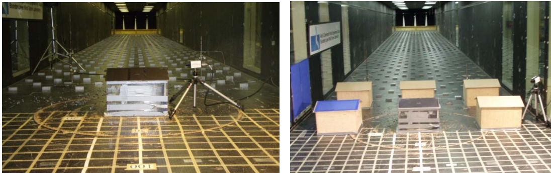
Figure 1. Photograph of the wind tunnel set-up looking upstream for (left) an isolated house in open country terrain, and (right) in a neighbourhood. The high speed camera is to the right of the house in order to obtain the video images of the initial failure and flight.
