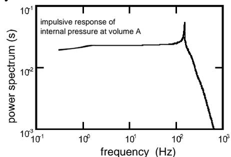
(b) Power spectrum of impulsive response of internal pressure at volume A evaluated by numerical model
