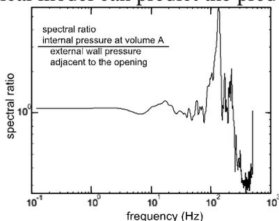
(a) Spectral ratio between internal pressures at volume C to wall pressures close to the opening (experimental)
