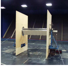
Figure 1: The sectional model on the dynamometric balance.
