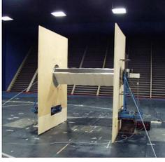
Figure 1: The sectional model on the dynamometric balance.
