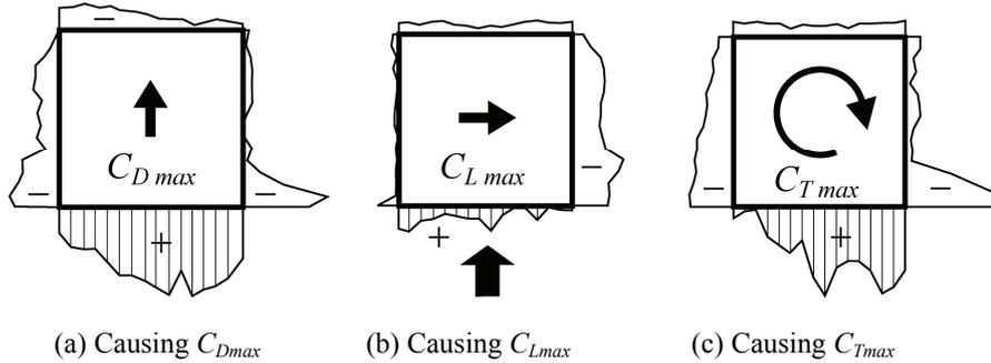
Figure 1: Examples of instantaneous pressure distributions causing maximum wind force coefficients for model LS ( $\alpha = 1/4$ ) [3]
