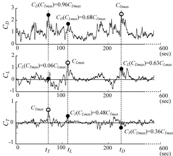
Figure 2: Maximum wind force component and accompanying other wind force components (LS) [3]
