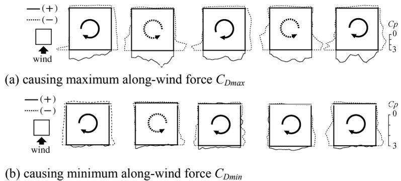
Figure 4: Instantaneous wind pressure distributions causing maximum /minimum wind force components ( $5H/8$ )
