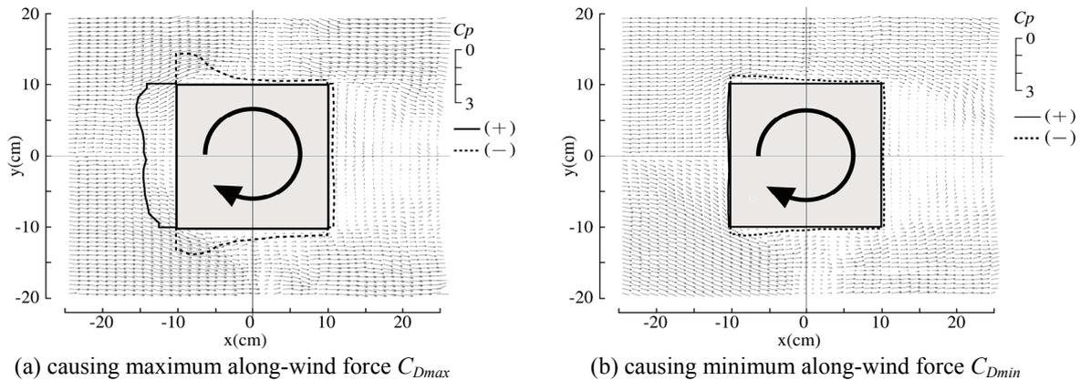
Figure 5: Ensemble-averaged instantaneous wind pressure distributions and flow fields causing maximum/minimum along-wind force components ( $5H/8$ )
