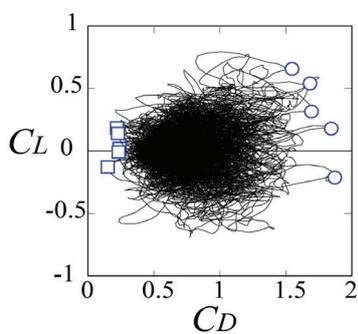
Figure 3: Phase-plane expression of wind force combination ( $C_D - C_L$ )
