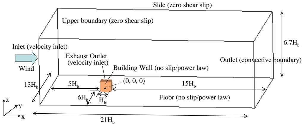
Figure 1: Computational domain and boundary conditions (LES).
