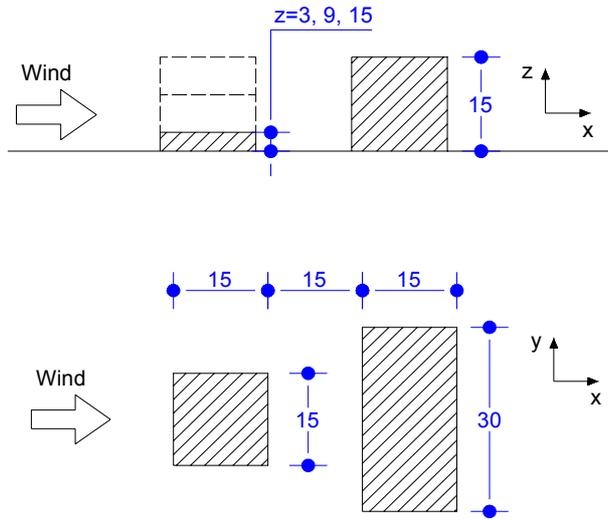
Figure 1: Sketch of the model, plane x-z and x-y.
