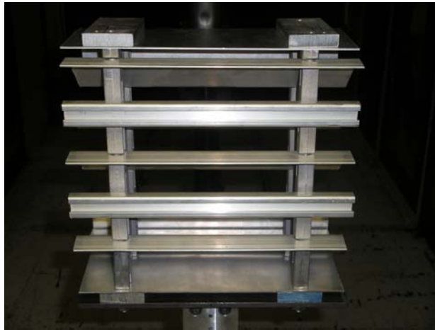
Figure 1: Aluminum louvered sign section as mounted in the tunnel
