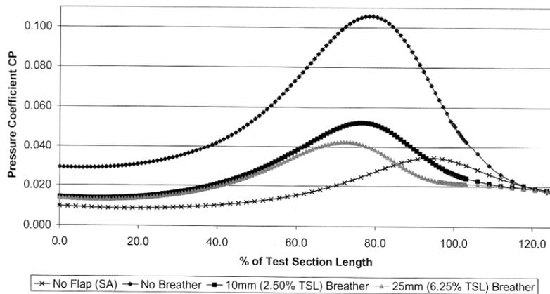
Figure 4. Effect of collector breather gap size on the predicted working section axial pressure distribution.
