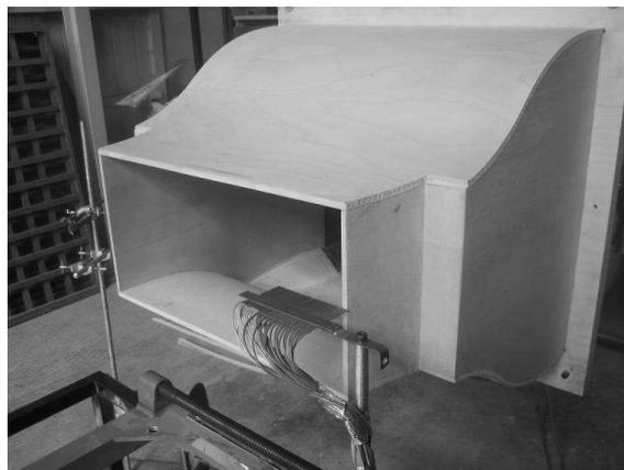
**Figure 2. View of 15% sub scale model of contraction with total pressure rake.**
