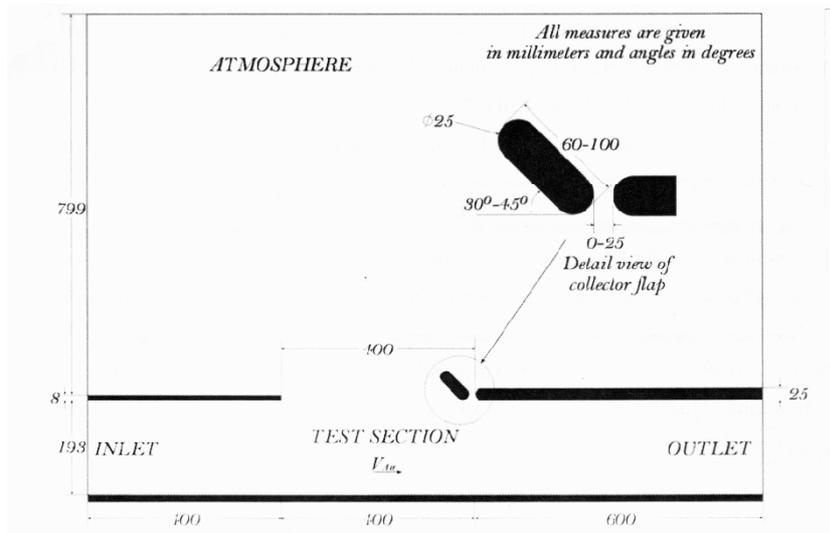
Figure 3. Arrangement of test section geometry used in the 2D CFD simulation
