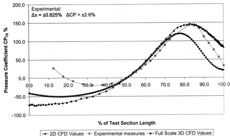
**Figure 5. Comparison of measured and CFD predictions of the working section axial pressure distribution.**
