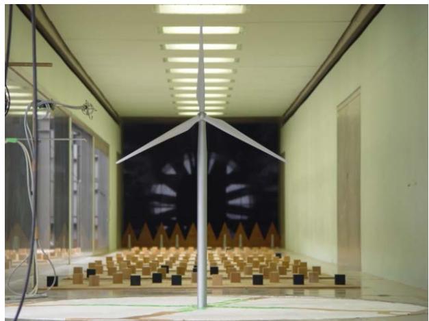
Fig.2 Model in the wind tunnel Blade pitch is 0 degree, Rotation of the blades is 0
