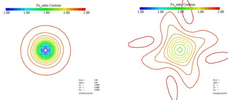
Figure 3: Pressure contour of a Rankine vortex after 1000 step. LSHUS(left) and Roe(right)
