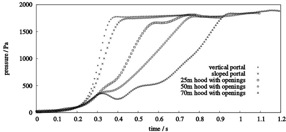
Figure 3: Entry pressure waves from different portal modifications
