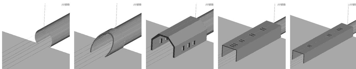
Figure 2: Portal modifications - from left: vertical portal ( $\eta = 1.08$ ), sloped portal ( $\eta = 0.75$ ), 25m hood ( $\eta = 0.47$ ), 50m hood ( $\eta = 0.26$ ), 70m hood ( $\eta = 0.34$ )
