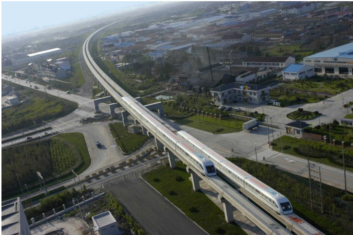
Fig. 1: Maglev vehicle Transrapid in Shanghai: Two vehicles passing each other at a relative speed up to 1000 km/h (image: Transrapid International)
