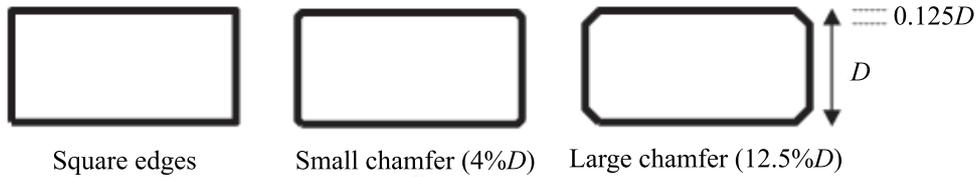
Figure 1: Cross-sections and edge configurations investigated
