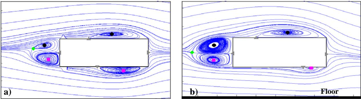
Fig. 1: Mean flow structures and critical points for the two cases considered: a)  $h_b/s=2.33$ , b)  $h_b/s=1$ . ●, anticlockwise vortex; ■, clockwise vortex; ▲, saddle on the obstacle surface; ◆, wake saddle.
