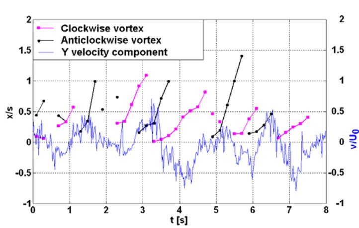
Fig. 4: Developing of the vortex structures and trend of the vertical component of velocity in point  $x/s=0.5$ ,  $y/s=0$ . Where  $v/U_0$  is the ratio between the vertical velocity component and the undisturbed mean velocity of flow upstream the obstacle.
