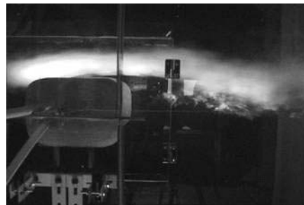
Fig.8: Visualized shear layer around the cylinder suppressed by jet.
