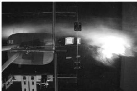
Fig.7: Visualized shear layer around the fixed cylinder.
