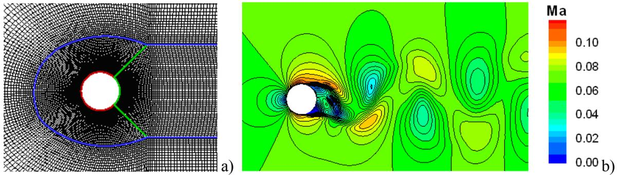
Figure 3: a) Grid distribution around a circular cylinder and b) Snap shot of the Mach number distribution past a fully rough circular cylinder. The Reynolds number is  $1 \times 10^6$  and the sand roughness height is  $kr=ks/D=450 \times 10^{-5}$ .
