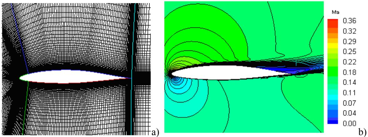
Figure 1: a) Grid distribution around the NACA65<sub>1</sub>-212 airfoil and b) Mach number distribution around the NACA65<sub>1</sub>-212 with 8% chord roughness near the leading edge. The Reynolds numbers is  $6 \times 10^6$ , the angle of attack is 11 degrees, and the sand roughness height is  $kr=ks/c=45.8 \times 10^{-5}$ .
