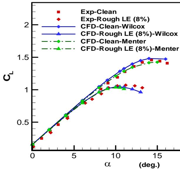
Figure 2: Lift coefficient versus the angle of attack for the NACA65<sub>1</sub>-212 airfoil with clean and rough configurations. The Reynolds numbers is  $6 \times 10^6$ , the angle of attack is 11 degrees, and the sand roughness height is  $kr=ks/c=45.8 \times 10^{-5}$ .
