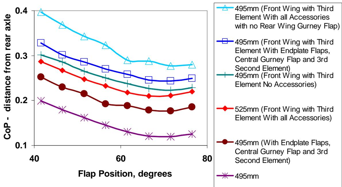
Figure 3: Rear wing height Effect on centre of pressure
