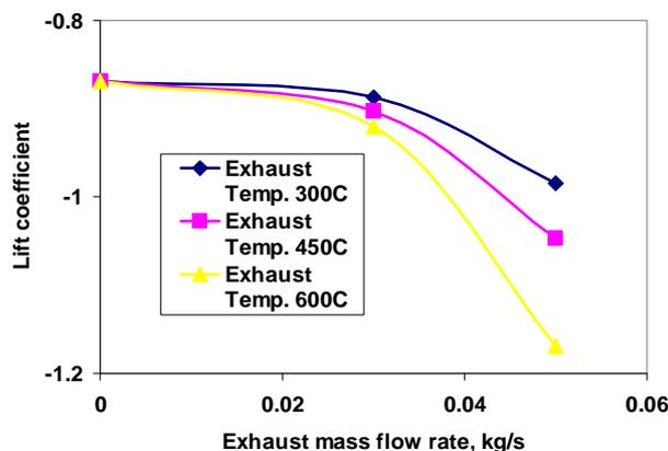
Figure 1: Effect of rear diffuser tunnel exhaust mass flow rate and gas temperature on the lift coefficient
