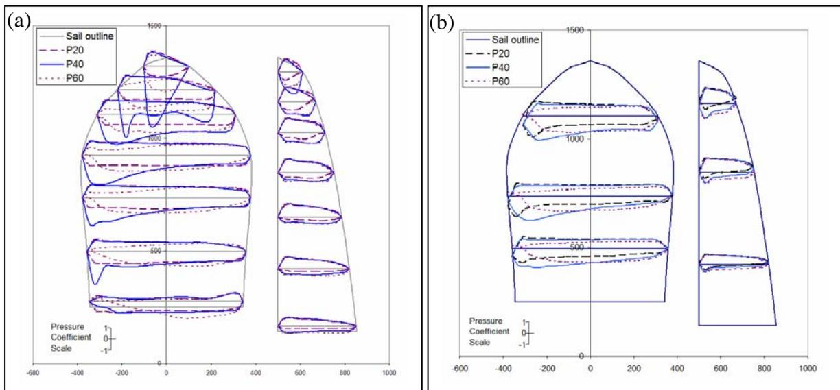
Figure 5: Pressures on the mainsail and spinnaker for three spinnaker pole angles ( $20^\circ$ ,  $40^\circ$  and  $60^\circ$ ) obtain from (a) wind tunnel testing and (b) CFD modelling. The boom was at  $75^\circ$  and the apparent wind angle  $120^\circ$ .
