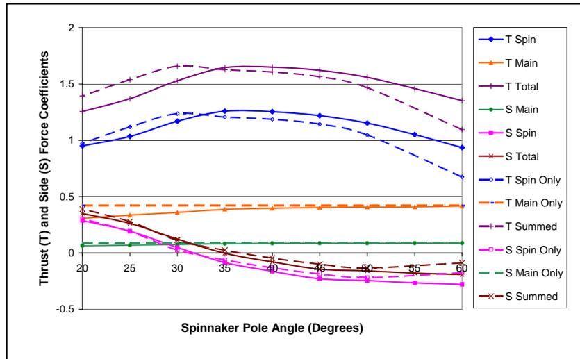
Figure 4: The effects of varying spinnaker angle when the boom is at  $75^\circ$  and the apparent wind angle  $120^\circ$ . Thrust and side forces on each sail as calculated by pressure integration from tests with the two sails together (solid lines) and independently (dashed lines).
