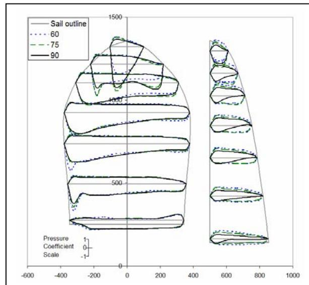
Figure 3: Pressures on the mainsail and spinnaker for three boom angles ( $60^{\circ}$ ,  $75^{\circ}$  and  $90^{\circ}$ ). The spinnaker pole was at  $40^{\circ}$  and the apparent wind angle  $120^{\circ}$ .
