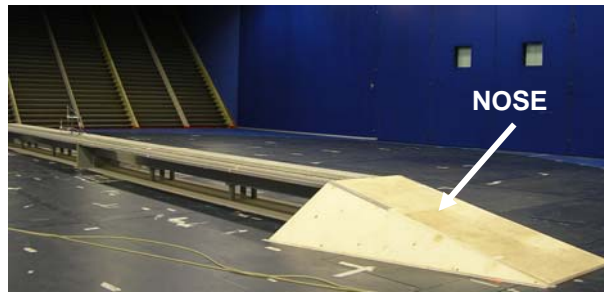
Figure 15. Viaduct with nose, characterization tests: cobra probe over the viaduct model (1:20 scale).
