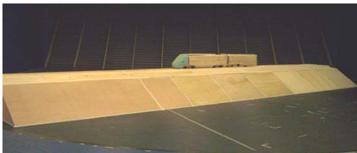
Figure 1. Experimental wind tunnel tests: 1:10 model of ETR500 on 6m high standard embankment.
