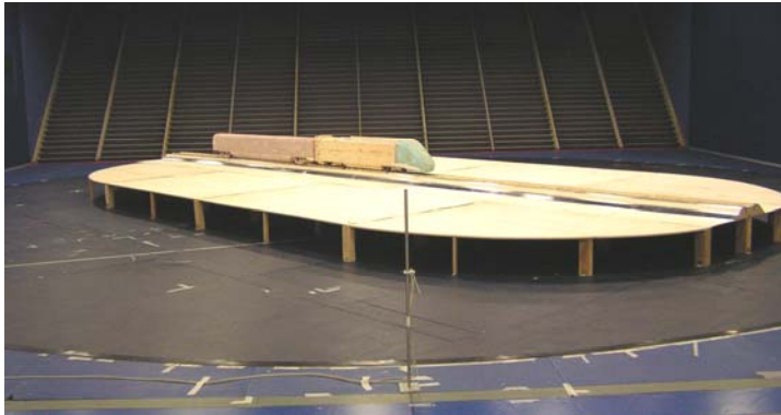
Figure 3. Experimental wind tunnel tests: 1:10 scale model of ETR500 on flat ground with ballast and rail.
