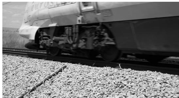
Figure 2 - Photograph of initial observations showing lightweight tapes attached to a metal bar on the trackbed shoulder during a Eurostar pass
