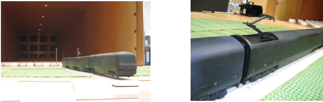
Figure 3: A 1:30 th scale model of a 4-car Class 365 EMU in the RWDI-Anemos wind tunnel
