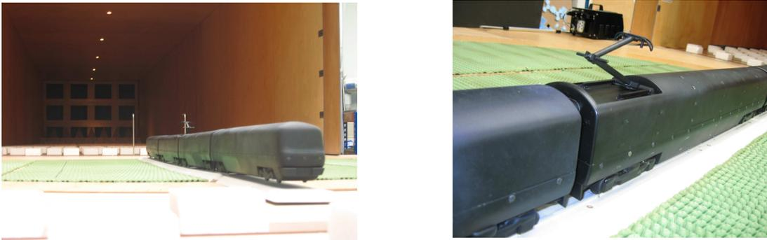
Figure 3: A 1:30<sup>th</sup> scale model of a 4-car Class 365 EMU in the RWDI-Anemos wind tunnel
