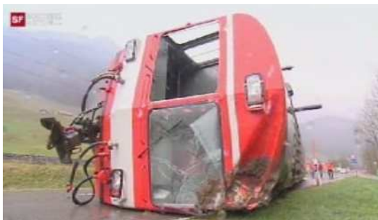
Figure 1: Train which turned over during winter storm Kyrill in January 2007, courtesy of Schweizer Fernsehen-Schweiz Aktuell
