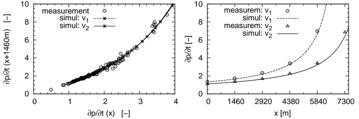
Figure 6: Wave-steepening prior to installation of absorbers: Left: Maximum pressure gradient (in arbitrary units) after propagation through a segment of length 1460 m. Right: evolution of the maximum pressure gradient along the tunnel for two train speeds  $v_1$  and  $v_2$ .
