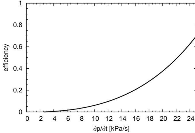
Figure 9: Efficiency of absorbers as function of the maximum pressure gradient of the compression wave. The horizontal axis can also be interpreted as characteristic frequency (in  $Hz$ ) of the wave.
