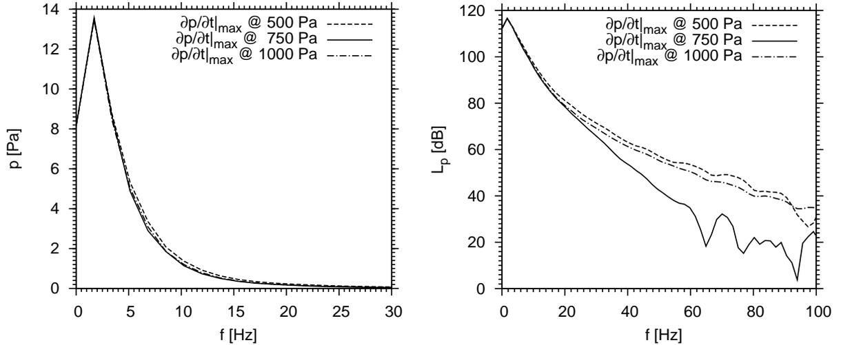
Figure 11: Power spectrum (periodogram) of the emitted pressure pulse after wave propagation for  $6000 m$  using  $\epsilon_{us} \approx 3$ . The signal was sampled with  $3500 Hz$  over  $0.5753 s$ .
