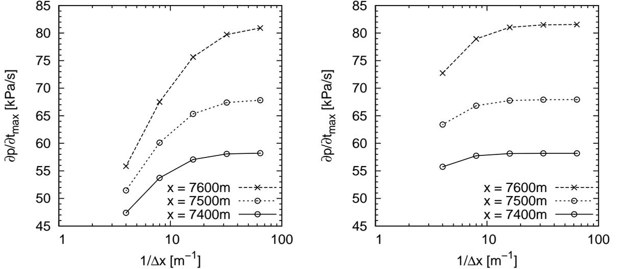
Figure 3: Dependence of the maximum pressure gradient on the spatial resolution  $\frac{1}{\Delta x}$  after propagation over 7400 m, 7500 m, and 7600 m for the McCormack scheme (left) and for the Godunov scheme (right).
