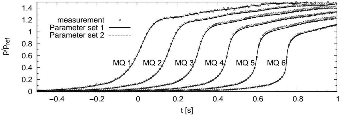
Figure 7: Comparison of measured and simulated compression wave (in arbitrary units) at six locations in the tunnel after installation of acoustical absorbers. Only a subset of the measurements is shown.
