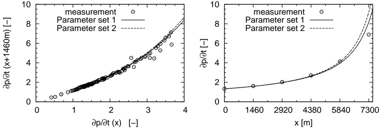
Figure 8: Comparison of wave-steepening after installation of absorbers for two sets of friction parameters. Left: Maximum pressure gradient (in arbitrary units) after propagation through a segment of length 1460 m. Right: evolution of the maximum pressure gradient along the tunnel.
