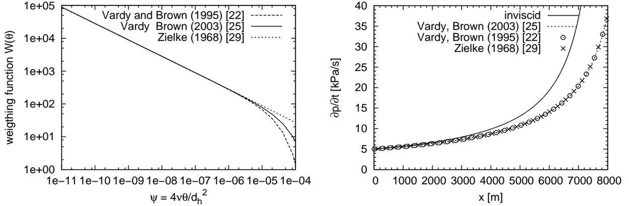
Figure 1: Comparison of three models for the unsteady friction term: Left: different approximations of the weighing function  $W$  as function of  $\theta = t - \tau$ , Right: evolution of the maximum pressure gradient in a simulation with  $\lambda = 0$ ,  $\epsilon_{us} = 5$ , and three models for  $W$ .
