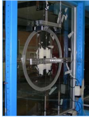
Figure 13: Lateral view of the elastic suspension system for the aeroelastic tests
