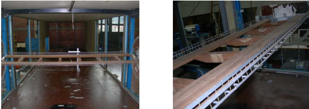
Figure 7: Section model tested in the CRIACIV wind tunnel
