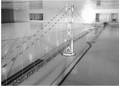
Photo1: Akashi Full-scale Model, 1/100 scale, 40m total span length (courtesy of Honshu-Shikoku)
