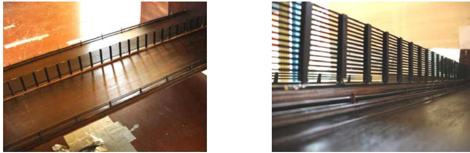
Figure 1. – Wind tunnel model of the viaduct Bukovo
