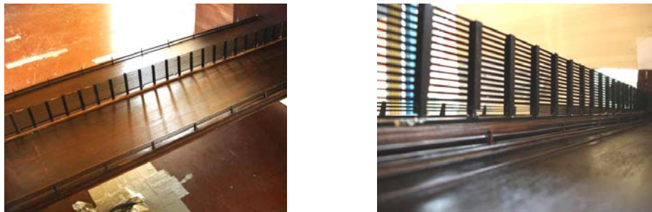
Figure 1. – Wind tunnel model of the viaduct Bukovo
