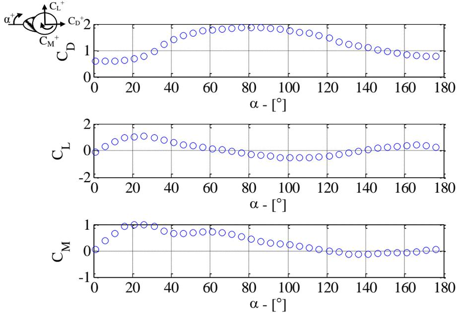
Figure 6. Aerodynamic coefficients taken from Ref. [2] and transformed into the model's coordinate system.
