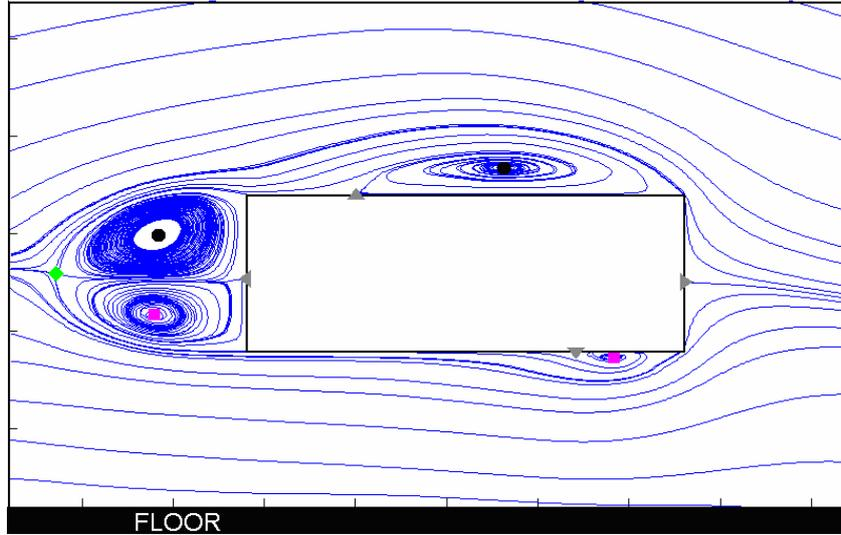
Fig. 3: Mean flow structure ( $h_b/s=1$ ,  $h^*=5$ ); ●, anticlockwise vortex; ■, clockwise vortex; ◆, ▲, saddle points.
