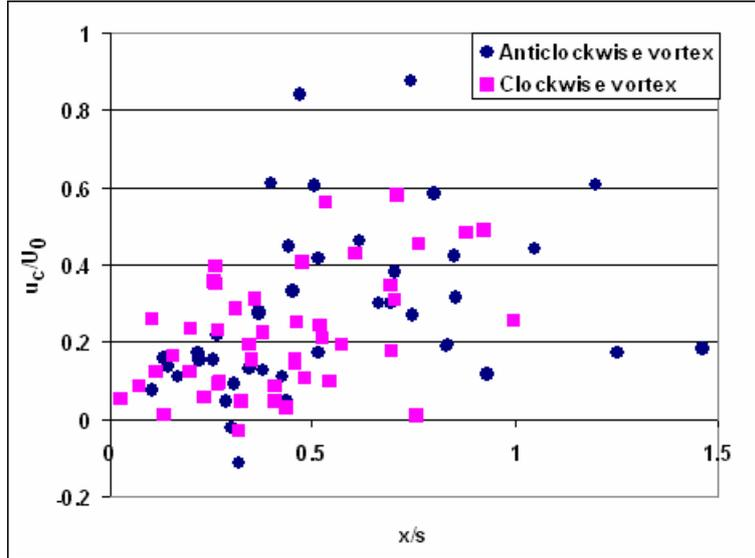
Fig. 14: Local convection velocity versus distance from the obstacle in the base region
