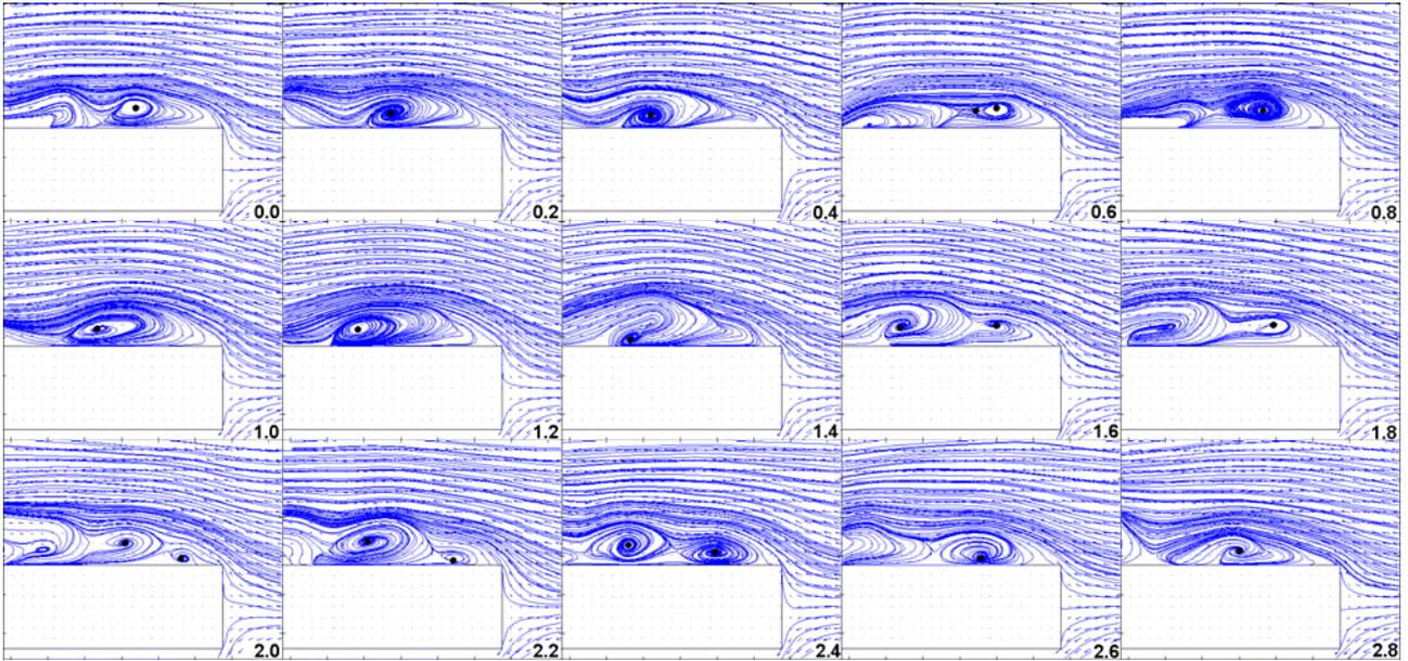
Fig. 7: Flow evolution in the extrados region,  $h_b/s=2.33$ ,  $h^*=5$ ,  $Re=1.2 \cdot 10^4$  (progressive time in seconds).
