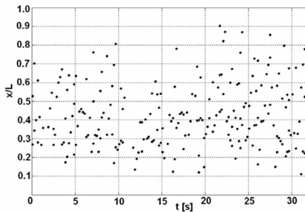
Fig. 8: Position of vortex centers along the rectangular cylinder versus time
