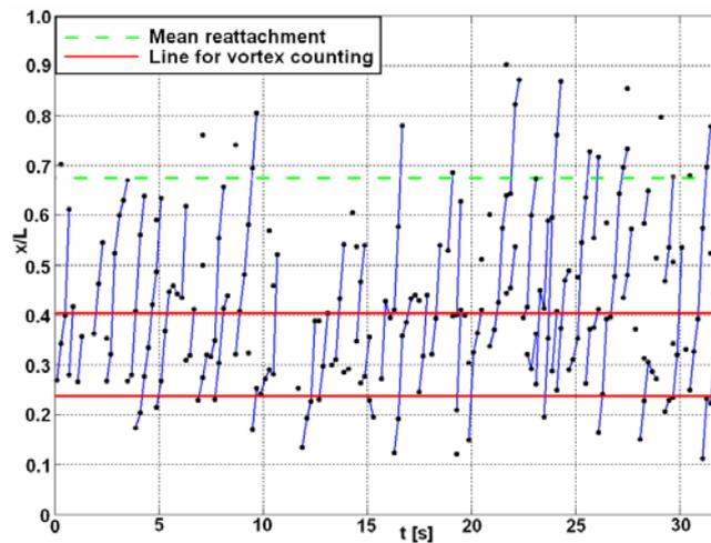
Fig. 10: Vortex center movements related to time. Lines for the calculation of the shedding frequency are reported.
