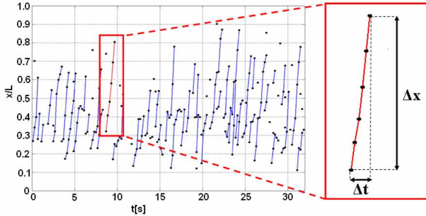
Fig. 9: Vortex center position related to time in the extrados region and calculation of convection velocity along a single trajectory,  $u_c = \Delta x / \Delta t$ .
