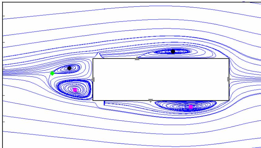
Fig. 2: Mean flow structures ( $h_b/s=2.33$ ,  $h^*=5$ ); ●, anticlockwise vortex; ■, clockwise vortex; ◆, ▲, saddle points.
