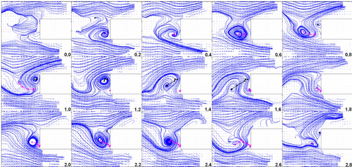
Fig. 11: Flow evolution of base region (progressive time in seconds)
