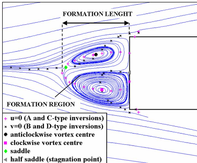
Fig. 6: Mean flow structures in the rear region;
