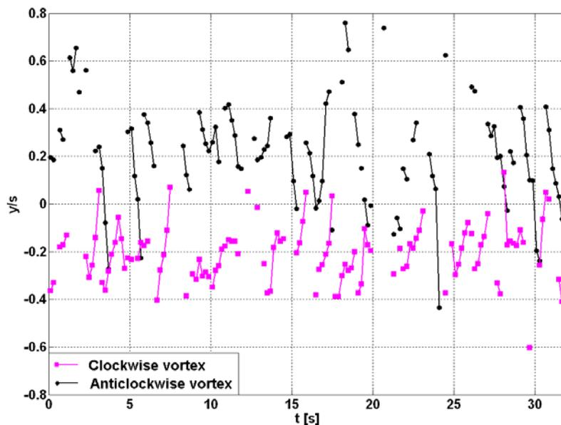
Fig. 13: Y movements of the vortex centres versus time.
