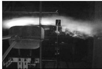
Figure 19: Visualized shear layer around the cylinder suppressed by jet.
