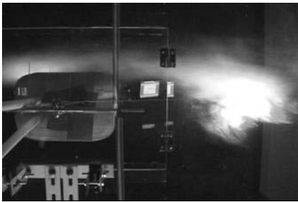
Figure 18: Visualized shear layer around the fixed cylinder.
