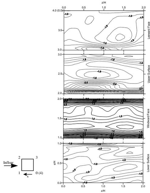
Figure 5. Instantaneous pressure at frame 5
