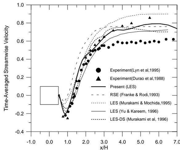
Figure 2. Time-averaged horizontal streamwise velocity along center
