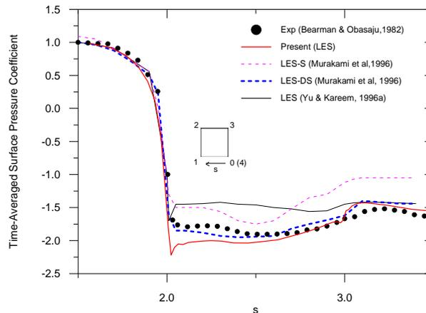
Figure 3. Time averaged pressure distribution on square cylinder
