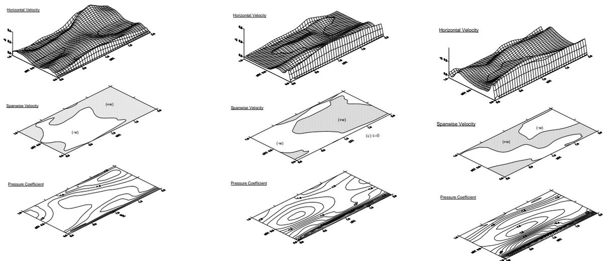
Figure 6. Instantaneous pressure and velocity on upper wall at frames 1, 3 and 5 from left
