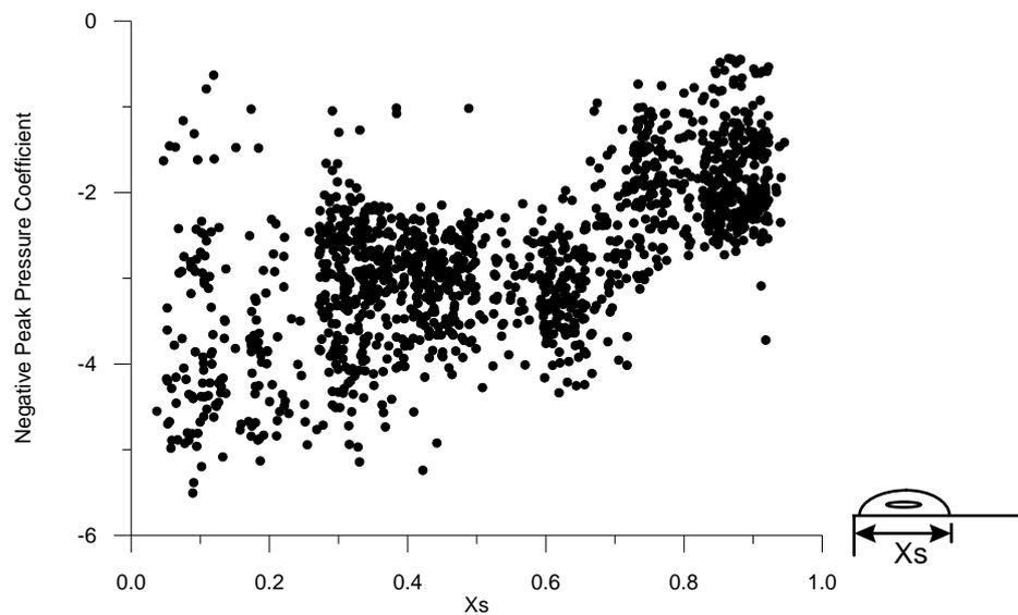
Figure 9. Scatter Plot of Negative Peak Pressure vs. Recirculation Length on Upper Wall of a Square Cylinder
