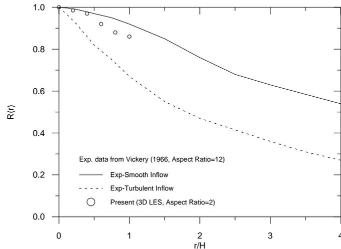
Figure 8. Spanwise Correlation Coefficients of Pressure Difference across Center Line of a Square Cylinder
