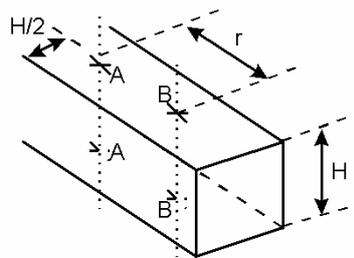
Figure 7. Schematic diagram for spanwise pressure correlation
