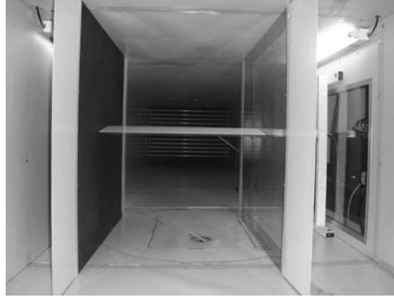
Figure 4: Rear view of the model and panels into the test section.
