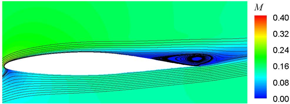
Figure 10: Mach number distribution around the airfoil with rough leading edge,  $\alpha=11^\circ$ , for  $M_\infty=0.14$ ,  $k_s/D=45.83\times 10^{-5}$  and  $Re_C = 6\times 10^6$  (steady state solution).
