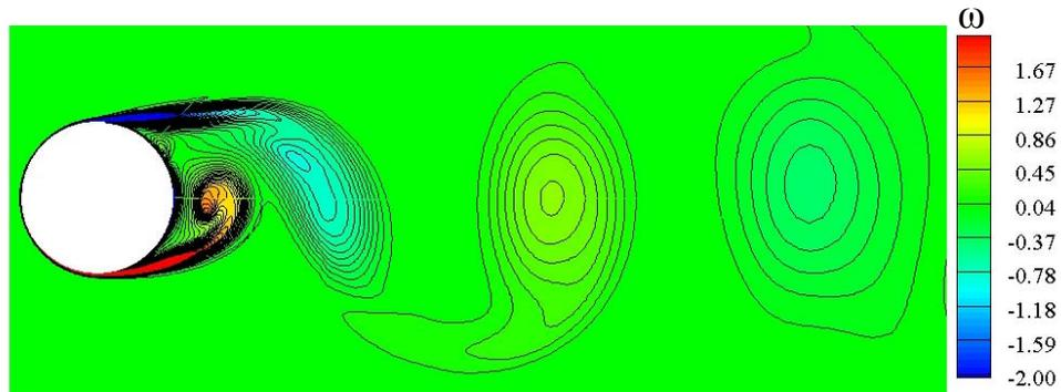
Figure 2: Snapshot of the flow vorticity contours around the rough circular cylinder and in the wake, using the modified Menter SST  $\kappa\text{-}\omega$  turbulence model, for  $M_\infty=0.07$ ,  $k_s/D=450\times 10^{-5}$  and  $Re_D = 10^6$ .
