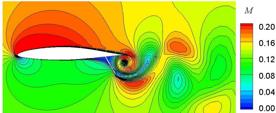
Figure 14: Snapshot of the unsteady flow past the clean leading edge airfoil with deployed flap, at  $\alpha=4^\circ$ , obtained with the modified Menter SST  $\kappa\omega$  turbulence model, for  $M_\infty=0.14$ ,  $k_s/D=45.83\times 10^{-5}$  and  $Re_C=6\times 10^6$ .
