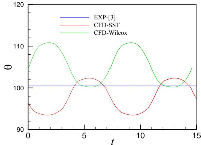
Figure 7: Separation angle over two periods of time, obtained with the Wilcox  $\kappa\omega$  and modified Menter SST  $\kappa\omega$  turbulence models, compared to the experimental data [3], for  $M_\infty=0.07$ ,  $k_s/D=450\times 10^{-5}$  and  $Re_D=3\times 10^6$ .
