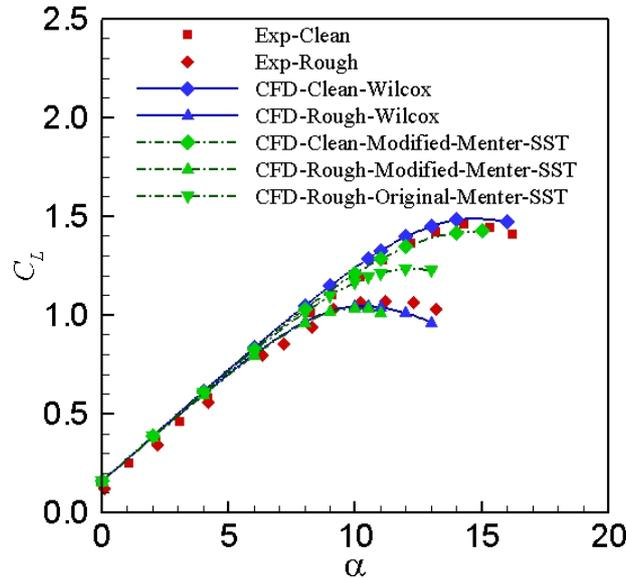
Figure 11: Lift coefficient versus angle of attack for the airfoil with clean and rough leading edges, for  $M_\infty=0.14$ ,  $k_s/D=45.83\times 10^{-5}$  and  $Re_C = 6\times 10^6$  (steady state solution).
