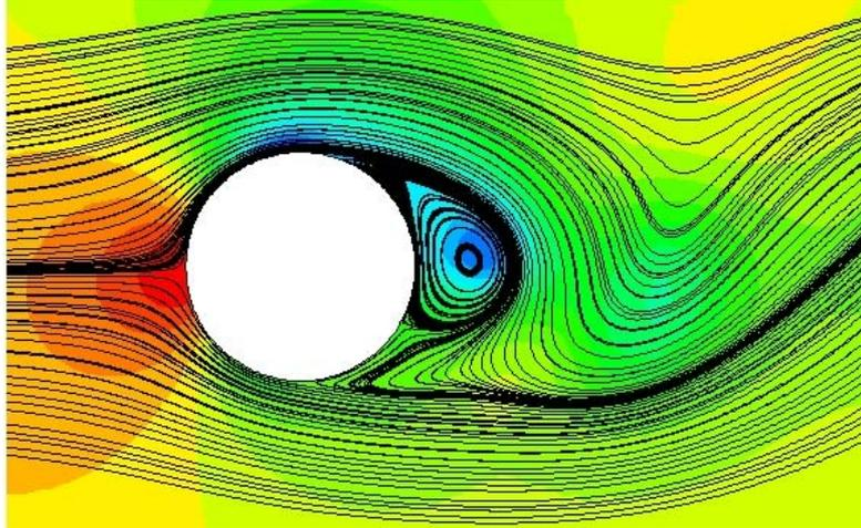
Figure 4: Snapshot of the flow streamlines and pressure distribution around the rough circular cylinder, obtained using the modified Menter SST  $\kappa\text{-}\omega$  turbulence model, for  $M_\infty=0.07$ ,  $k_s/D=450\times 10^{-5}$  and  $Re_D = 10^6$ .
