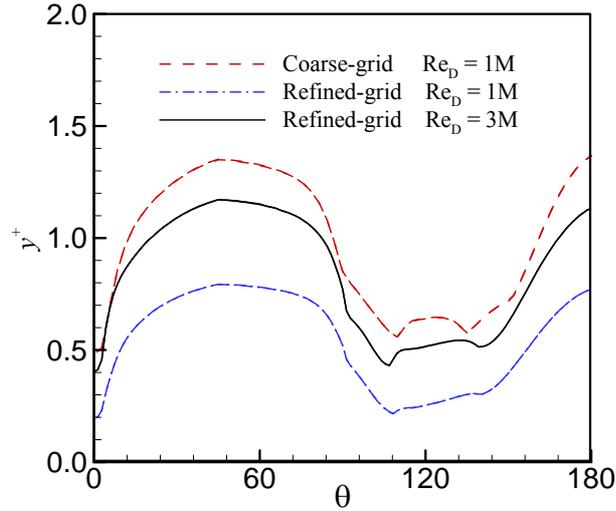
Figure 5: Time averaged  $y^+$  profile around the rough circular cylinder for coarse and refined grids at  $Re_D = 1 \times 10^6$  and  $3 \times 10^6$ , using the modified Menter SST  $\kappa\omega$  turbulence model.
