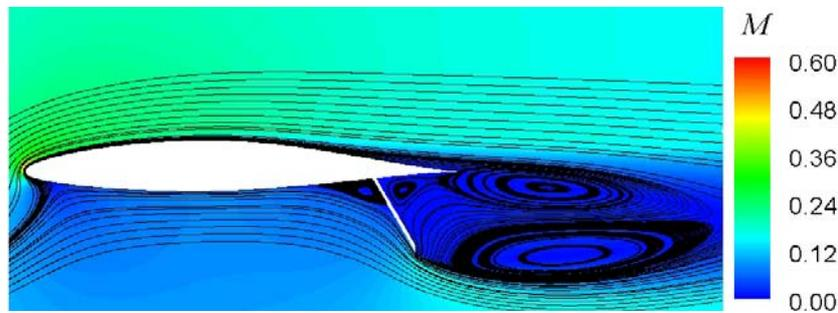
Figure 12: Mach number distribution and streamlines around clean leading edge airfoil with deployed flap, at  $\alpha=9.5^\circ$ , obtained with the modified Menter SST  $\kappa\omega$  turbulence model, for  $M_\infty=0.14$ ,  $k_s/D=45.83\times 10^{-5}$  and  $Re_C = 6\times 10^6$  (steady state solution).
