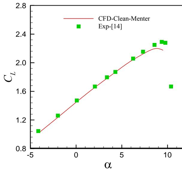
Figure 13: Lift coefficient versus the angle of attack for clean leading edge airfoil with deployed flap, obtained with the modified Menter SST  $\kappa\omega$  turbulence model, for  $M_\infty=0.14$ ,  $k_s/D=45.83\times 10^{-5}$  and  $Re_C = 6\times 10^6$  (steady solution).
