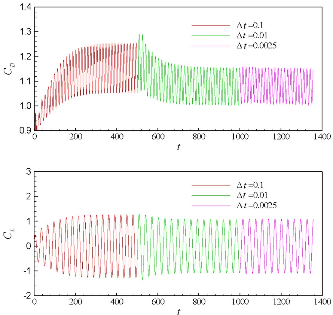
Figure 3: Time-history of the predicted drag ( $C_D$ ) and lift ( $C_L$ ) coefficients for a rough circular cylinder, obtained with the modified Menter SST  $\kappa\text{-}\omega$  turbulence model, for  $M_\infty=0.07$ ,  $k_s/D=450\times 10^{-5}$  and  $Re_D = 10^6$ .
