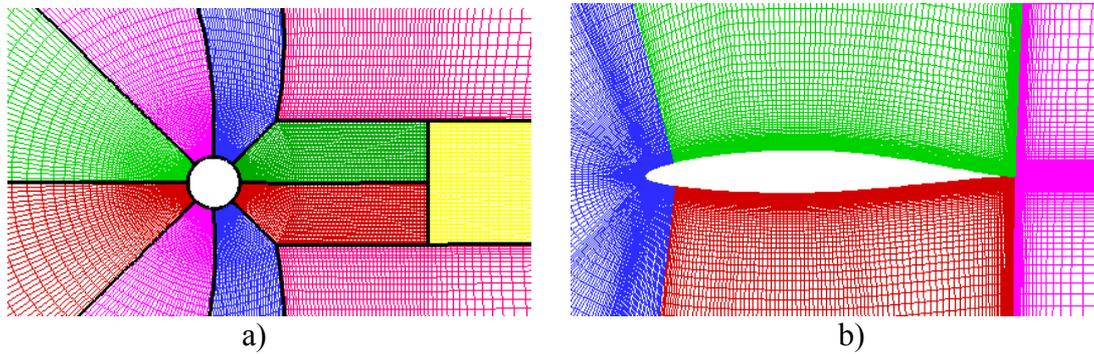
Figure 1: Grid distribution: a) around a circular cylinder, b) around an airfoil.
