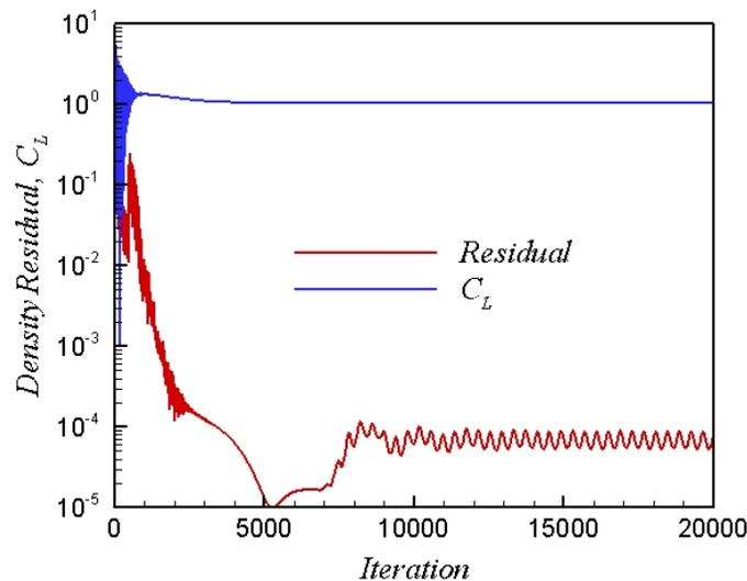
Figure 9: Lift coefficient and density residual history for the airfoil with rough leading edge, for  $\alpha=11^\circ$ ,  $M_\infty=0.14$ ,  $k_s/D=45.83 \times 10^{-5}$  and  $Re_C = 6 \times 10^6$  (steady state solution).
