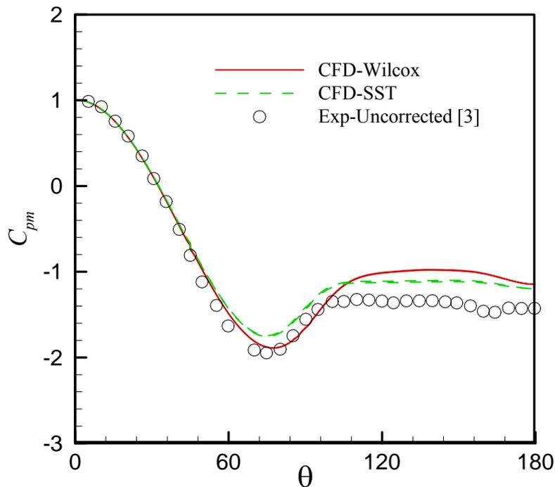
Figure 6: CFD time-averaged pressure coefficient profile on the rough circular cylinder at  $Re_D=3\times 10^6$ , obtained with the Wilcox  $\kappa\text{-}\omega$  and modified Menter SST  $\kappa\text{-}\omega$  turbulence models, compared to the uncorrected measured data [3], for  $M_\infty=0.07$ ,  $k_s/D=450\times 10^{-5}$  and  $Re_D=3\times 10^6$ .
