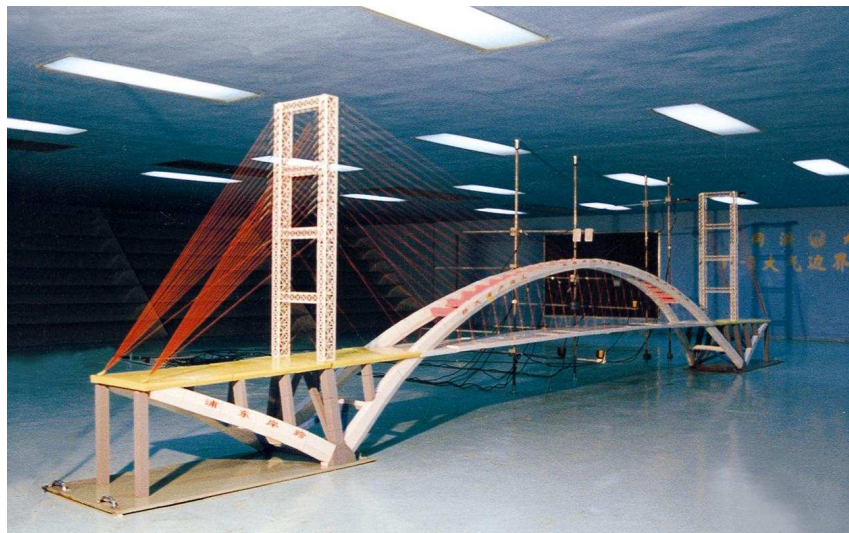
Figure 14: Aerodynamic model of Shanghai Lupu Bridge
