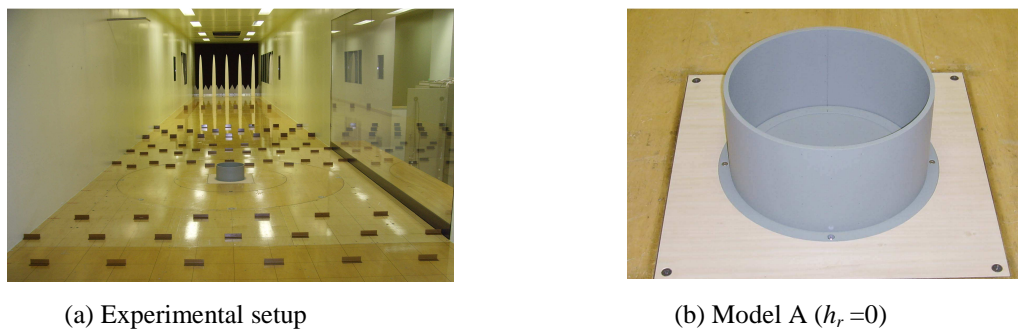
Figure 1: Experimental setup and model for pressure measurements (Model A).
