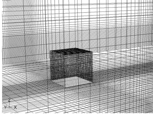
Figure 1: 3D mesh around a cube mounted on a surface
