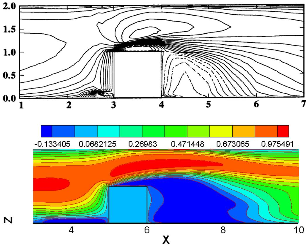
Figure 8: Time-averaged streamwise velocity contours on the symmetry plane. Figure on top is the experimental result of Martinuzzi and Tropea (1993); bottom is the result from LES
