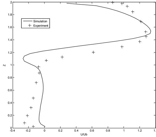
Figure 7: Time-Averaged streamwise velocity at  $x=6.08H_b$
