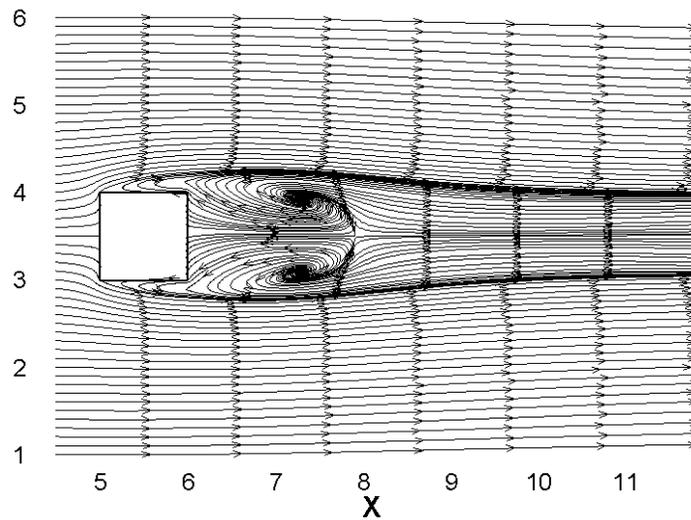
Figure 12: Time-averaged streamlines of flow past a cube in channel at the cube centerline Horizontal plane
