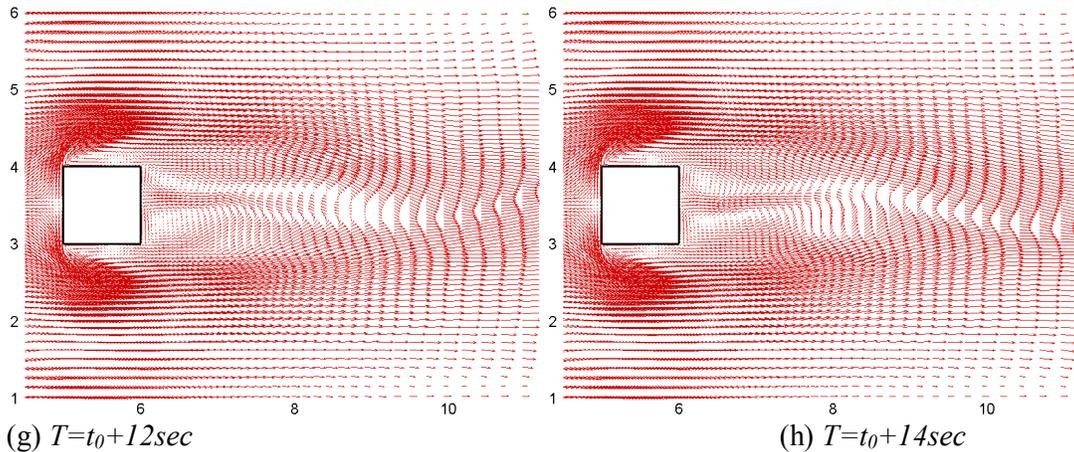
Figure 13: Instantaneous velocity vectors at the horizontal plane through the centerline of the cube at different time steps
