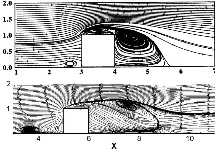
Figure 9: Time-averaged streamlines on the symmetry plane. Figure on top is the experimental result of Martinuzzi and Tropea (1993); bottom is the result of the present code
