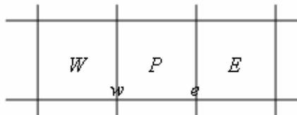
Figure 2: grid notations in the  $x$ -direction
