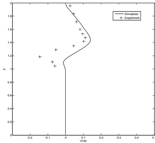
Figure 11: Time-Averaged  $y$ -component of velocity at  $x=5.75H_b$
