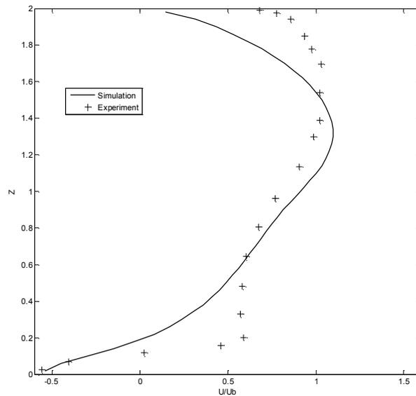
Figure 4: Time-Averaged streamwise velocity at  $x=4.68H_b$
